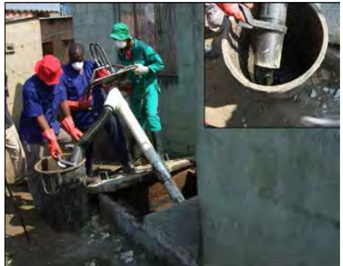
Field testing in Durban, South Africa showed the ability of the extraction auger in emptying pit latrines as a portable, hygienic technology. The testing also showed the high variability of pit latrine contents with respect to viscosity, water content, shear strength, and amount of trash.
