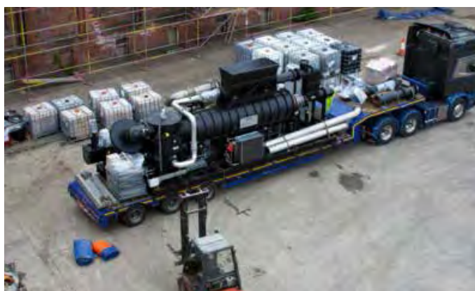
The pyrolysis unit and the pre-treatment units will be transportable on shipping containers. The pyrolysis unit can be delivered in two 40 ft shipping containers. Water treatment and dewatering units are currently in design.
