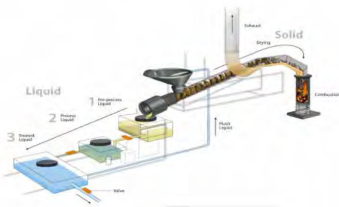
This figure shows the core steps in RTI’s integrated waste treatment system—auger-based solid liquid separation, liquid waste treatment via electrochemical disinfection, recycled liquid used for flush/rinse, and solid waste combustion (source for thermoelectric energy generation). Not shown is the Roca-designed squat plate.
