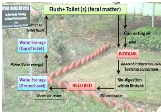
The flow diagram represents the complete cycle of our system. The fecal matter enters to Biotank through inlet pipe. After biodegradation and secondary treatment, water may be stored for reuse. Background photo: installed system at DRL gate where reuse of water for flushing is done.
